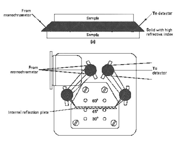
The above is a figure of attenuated total reflectance. Notice that the light bounces back forth in the sell. The idea is the principle of Snells law: the reflection occurs because the beam of radiation is passing <u>less</u> <u>dense to a more dense/more dense to a less dense</u> medium. Also <u>decreasing/increasing</u> the angle of the incident beam of radiation increases the fraction of radiation that is reflected.
